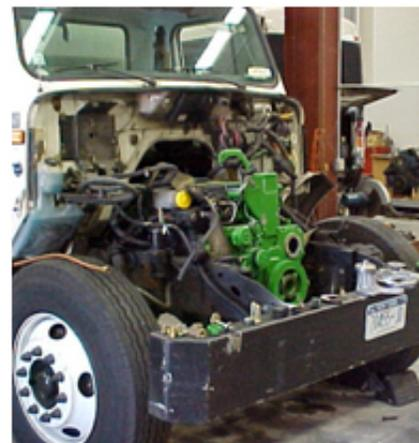
John Deere compressed natural gas engine used to re-power Manhattan Beer delivery trucks
