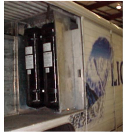
Compressed natural gas tanks installed on Manhattan beer trucks
